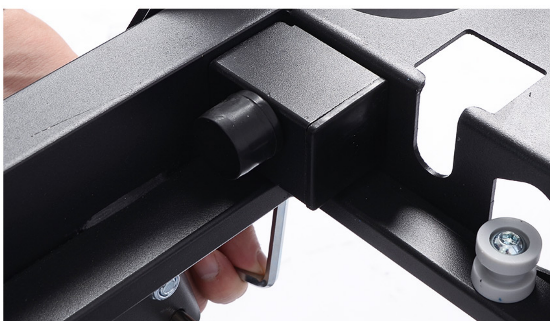
29. Use a small hex wrench to tighten the bolt.
