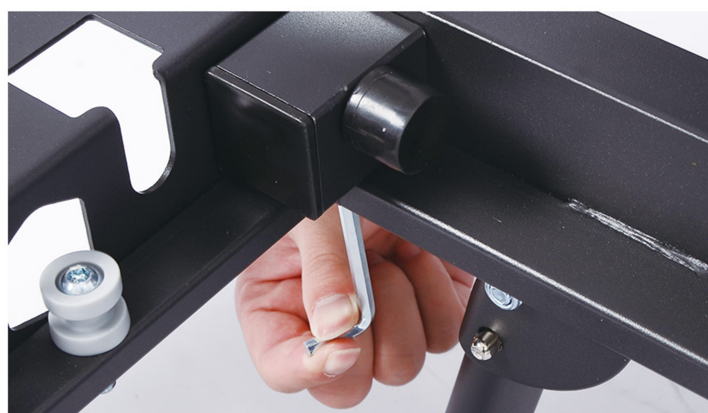
28. Use a small hex wrench to tighten the bolt.
